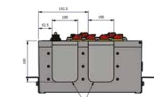
SLIDING DRILLABLE GLAND PLATE FOR MAIN IN/OUT SUPPLY
