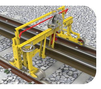
The rail borne trolley runs on profiled, flanged steel wheels which provide low friction, therefore minimising the force required to propel it. All handles and controls have been specifically designed to minimise the effort required for operation.
